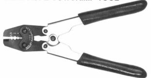
This three cavity, two jaw compound action tools is designed to provide clean, sharp cuts. It also crimps compression sleeves for loop and cap splices in a range of small wire rope sizes. The jaws are high carbon heat treated steel with the cutting blade induction hardened for maximum cutting life.
