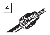
Align seal with wire insulation
