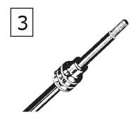
Apply correct seal per wire gauge size. Slide back seal to enable removal of insulation
