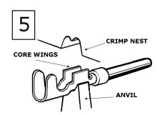
Core wings should be crimped first. Select the appropriate tool and appropriate cavity. (See tool matrix) Lay the back of the terminal core wings on the appropriate tool anvil. Be sure the core wings are pointing towards the crimp nest.
