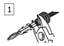
Cut off terminal between core and insulation crimp.
