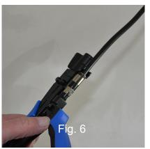
Squeeze the handles to compress the connector and coaxial cable. (Fig. 7)
