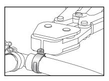
Fig. 1: Correct jaw tip placement
