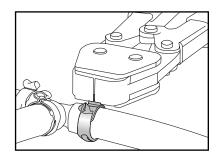
Fig. 3: Cut and remove clamp
