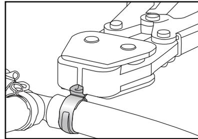
*Fig. 1: Correct jaw tip placement*
