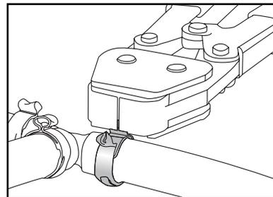
*Fig. 3: Cut and remove clamp*
