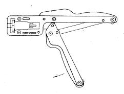
Install the un-compressed connector and cable by inserting the coax conductor into the hole in the compression tip.
