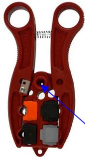
Insert 6/59 cable into the nest. Push down into nest and rotate back and forth between fingers.
