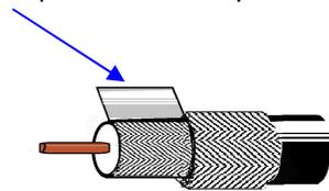
Fold back second layer of braid exposing foil covered foam core.
