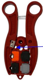
Insert 6/59 cable into the nest. Outer insulation should be flush to tool body. Rotate tool one or two revolutions
