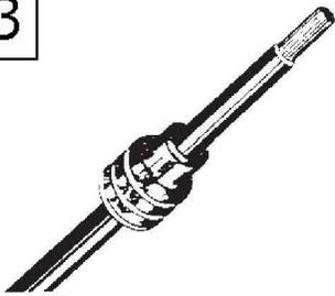
Apply correct seal per wire gauge size. Slide back seal to enable removal of insulation
