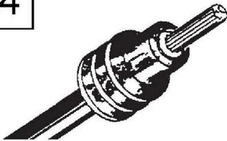
Align seal with wire insulation
